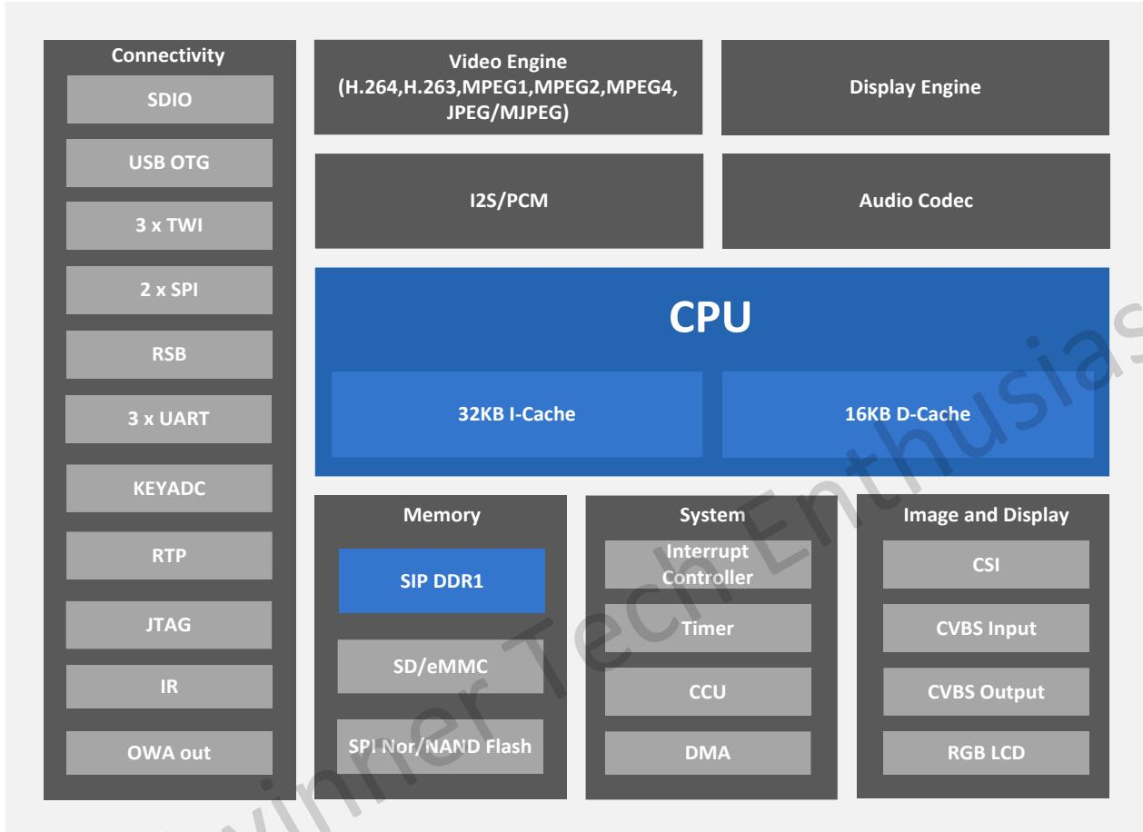
The typical application diagram of F1C200s is as follows:
